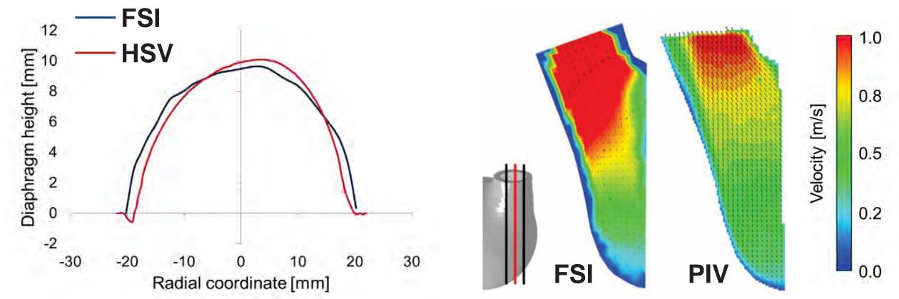
**Conclusions.** The developed FSI model can elucidate the continuous, timedependent and three-dimensional pVAD fluid dynamics as well as the threedimensional and asymmetric kinematics of the pVAD diaphragm. This approach may be pivotal in the optimization of the device, complementing ground truth data from PIV and HSV mock-loop *in-vitro* tests.
