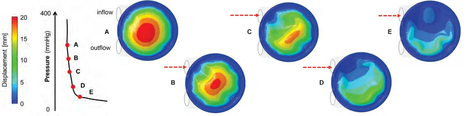
Fig. 2 Diastolic contour maps of pVAD nodal displacement along the normal direction to the diaphragm plane.
